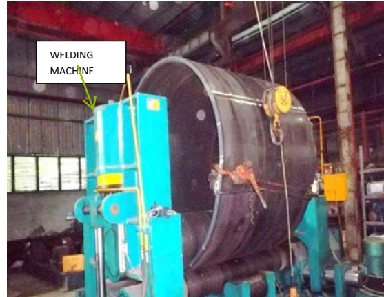
Figure 66 Preparation of boiler drum (Courtesy of Enertech-Philippines) (27)
