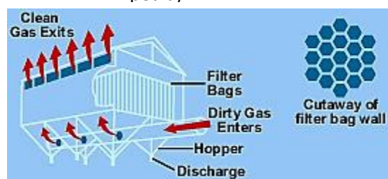
Figure 14 Fabric filter components (US-EPA) (94)
