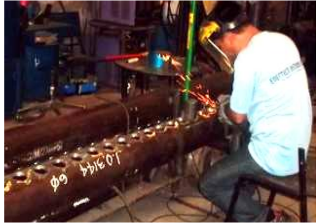
Figure 69 Heat exchanger header manufacturing (Courtesy of Enertech–Philippines)
